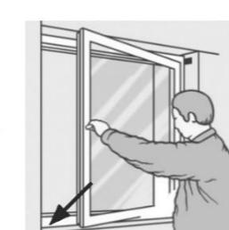
**UK:** Check that the sash on the opening side contacts the frame striking plate at the bottom. There should be gentle contact without having to exert excessive force. Adjust as necessary.
