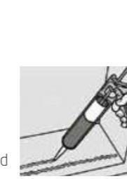
**UK:** Use a hardening mastic in two runs between the threshold and the base over the whole length.
