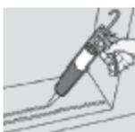
**UK:** Use hardening mastic in two runs between the threshold and the base over the whole length.
