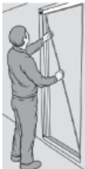
**UK:** Frame jambs must be square and plumb in both directions and the diagonals should be identical.
