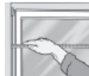
**UK:** Check the rebate widths are equal across the hinge and locking points.
