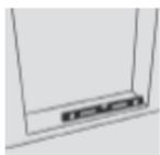
**UK:** Base under threshold must be flat and level. The entire depth of the threshold must be supported. See also section A-A.
