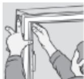
**UK:** Wedge the sides of the frame at the top with temporary double wedges. Check with a long spirit level that the frame sides are plumb and square. Check levels and fixings. Refit the door and re-fasten all the screws checking that fixings are the correct distance apart.
